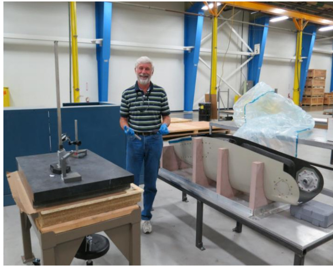
Pictured above - A [not usually] bearded Jay Watson dons blue elastic gloves to validate critical dimensions and prepare shipment on the first composite test and 'fit-up' Flap Track Fairing, a component of a pre-production demonstrator wing.
